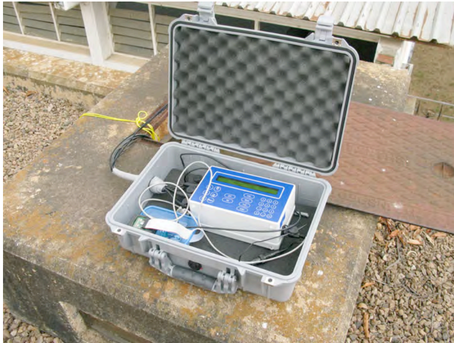
Fig. 4: A wireless sensor measuring water quality in Blantyre, Malawi.
